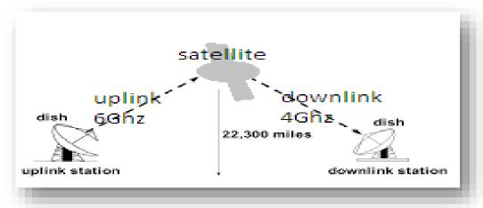
It support Very Long Range Communication with Line of Sight Propagation . It Cannot Penetrate Solid Objects. It is Very Expensive communication mode.
